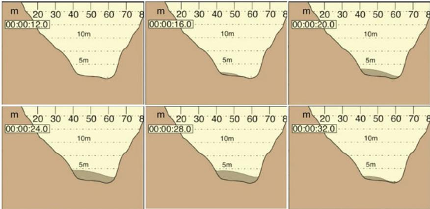
**Fig. 36.7** Total height of flowing after 1, 2, 3 and 4 min of simulation at an East–West section in point 1 in Fig. 36.6, close to the Abbey
