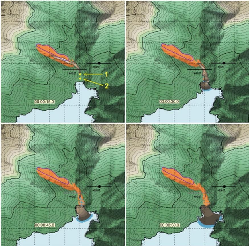
**Fig. 36.6** The simulation at 4 different time steps and the location of the section (2) in Fig. 36.7 and in Table 36.2 (1, 2)
