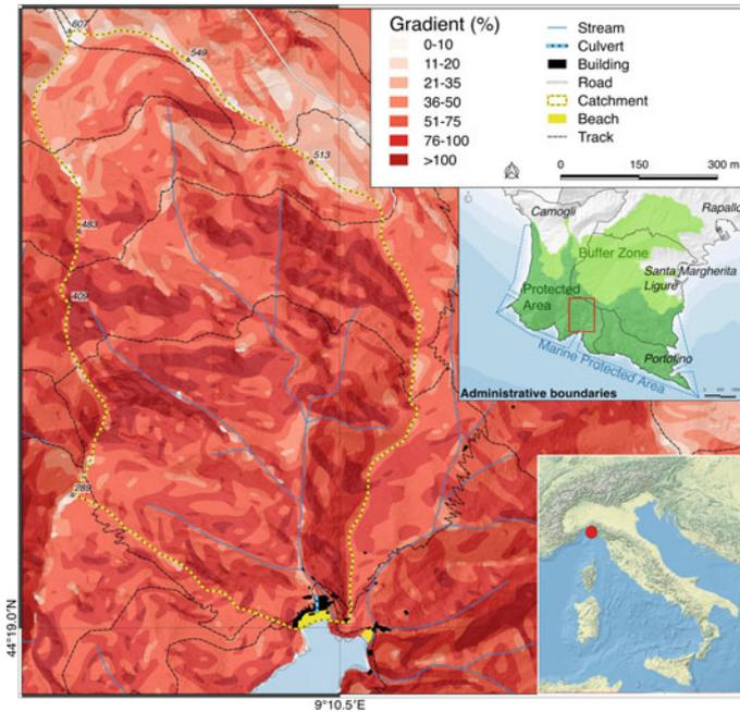
**Fig. 36.1** The San Fruttuoso catchment slope gradient, buildings and the culvert under the ancient Abbey, which flows on the small beach
