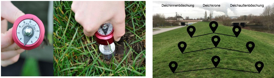
Assessment of shear stress using the pocket device (left) and the scheme for assessment (right) as a part of the risk based maintenance strategy of green dikes
