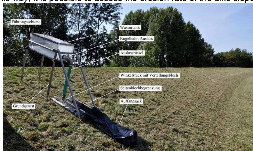
Figure 13 A innovative portable device “dike elephant” to assess the erosion stability of the green dikes as a part of the risk based maintenance strategy, developed at TUHH
