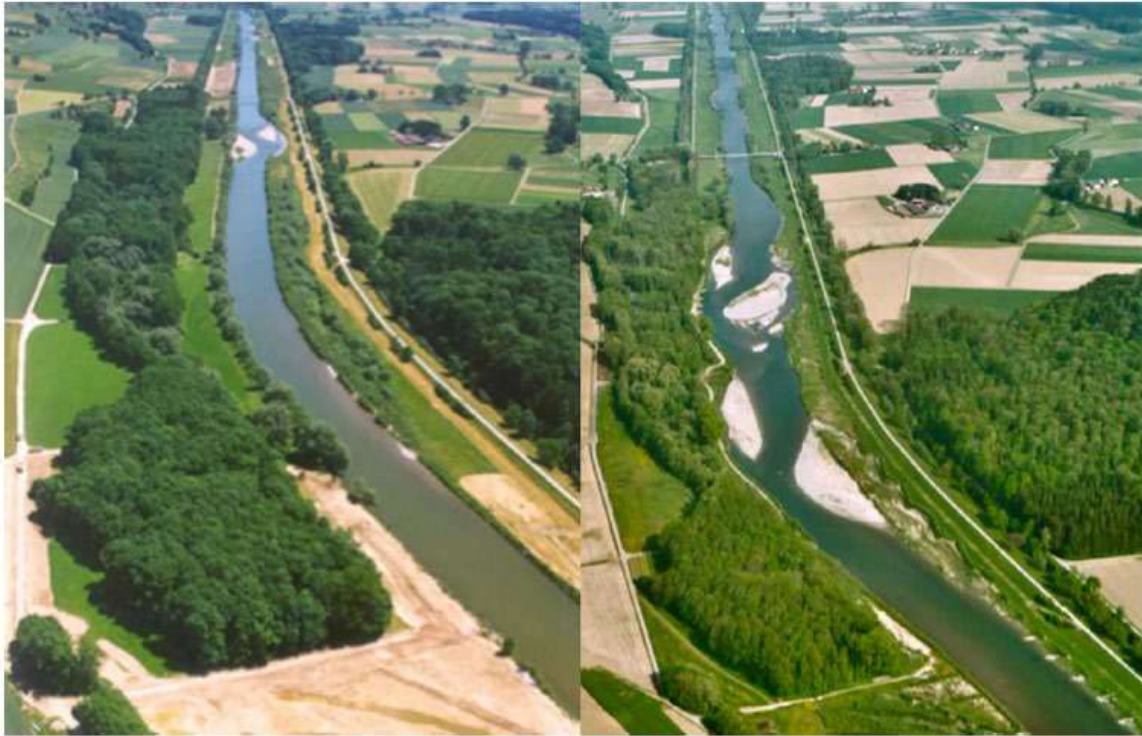
Figure B.27 Condition at the Thur section (left) before and (right) after the restoration (Source: Seidl and Stauffacher, 2013).
