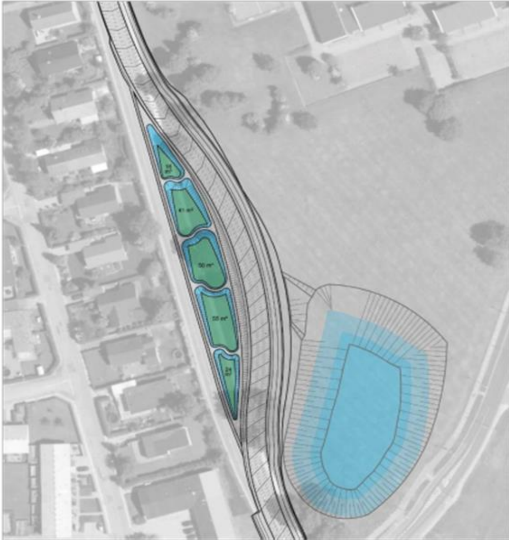
Figure 7-5 Lystrup Centervej sith waterpond, rain beds and changed road profile
