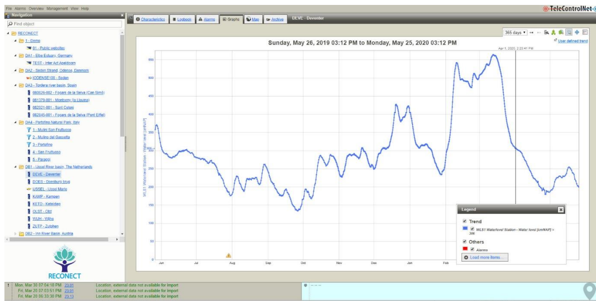
Figure 8.2 Example of historical monitoring data of water level at Deventer station in IJssel River, the Netherlands (DB1)
