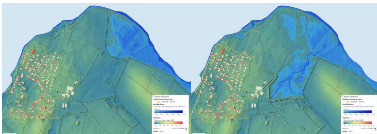
Figure 23: Flooding at 0,8-meter AMSL before (left) and after (right) the implementation of the NBS (Kildahl Sønderby, 2024).
