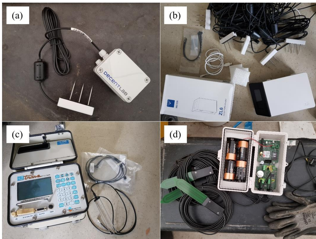
Figure 3: (a) TEROS-12 + Decentlab Datalogger + SENS (b) TEROS-11 + ZL6 Datalogger + ZENTRA Cloud (c) TDR (d) SMT100 + TrueLog100 Datalogger
