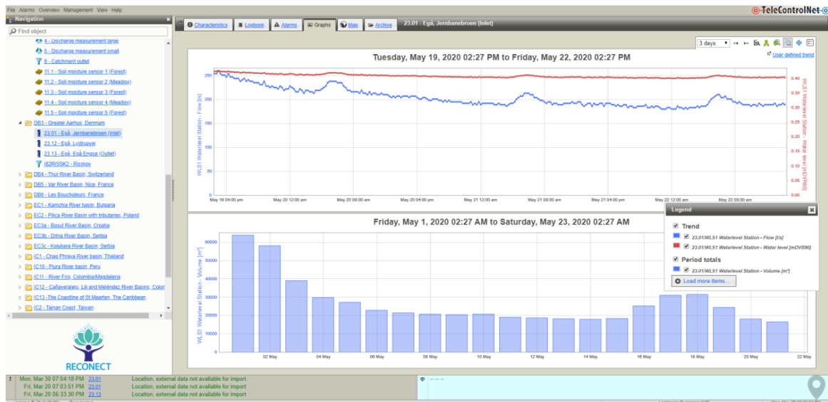
Figure 10: Example of monitoring data (water levels and retention volume) at Ega, Jernbanebroen (Inlet), Greater Aarhus, Denmark (DB3)
