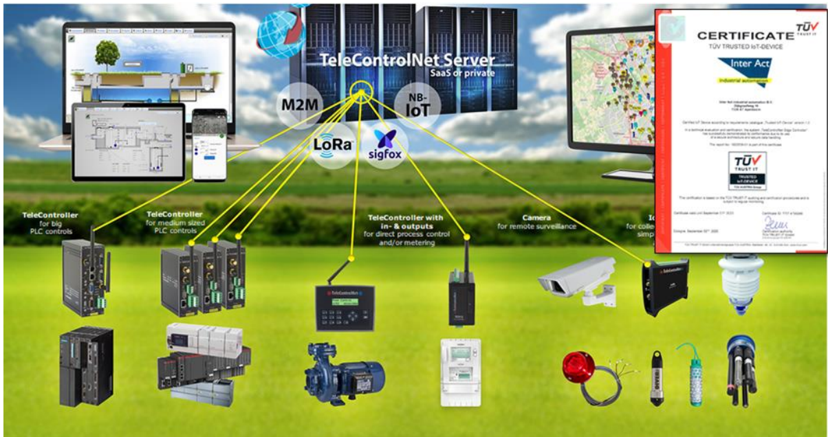
Figure 4. The TeleControlNet concept with edge controllers
