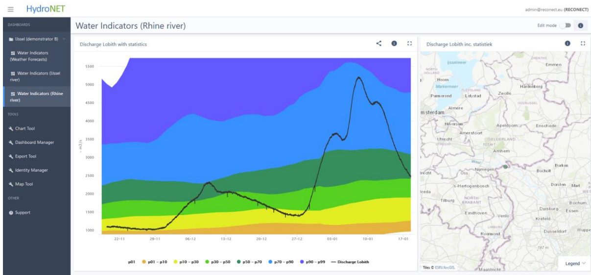
Figure 20 HydroNET platform dashboard for water managers in the IJssel demonstrator site. Dashboard shows the water level of the Rhine as it enters The Netherlands. The waterlevels are compared to 100-year statistics.
