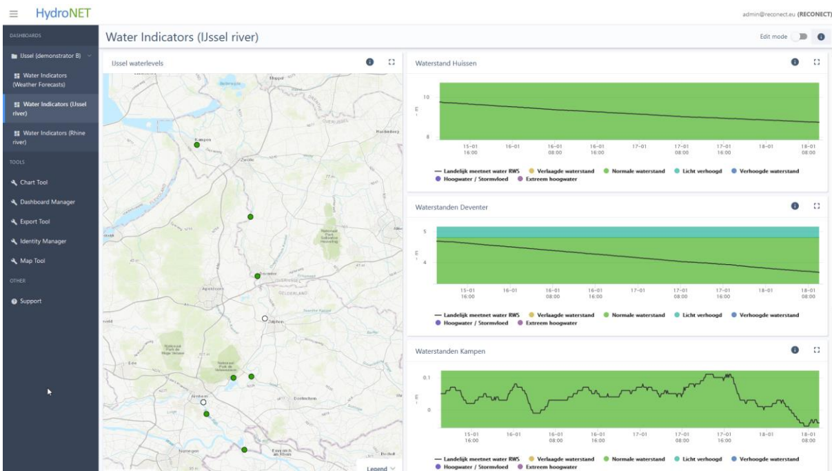
Figure 19 HydroNET platform dashboard for water managers in the IJssel demonstrator site. Dashboard shows the water level at multiple locations in the IJssel river. Each location is color coded, giving the water managers of the IJssel case a direct overview of the state of the river.
