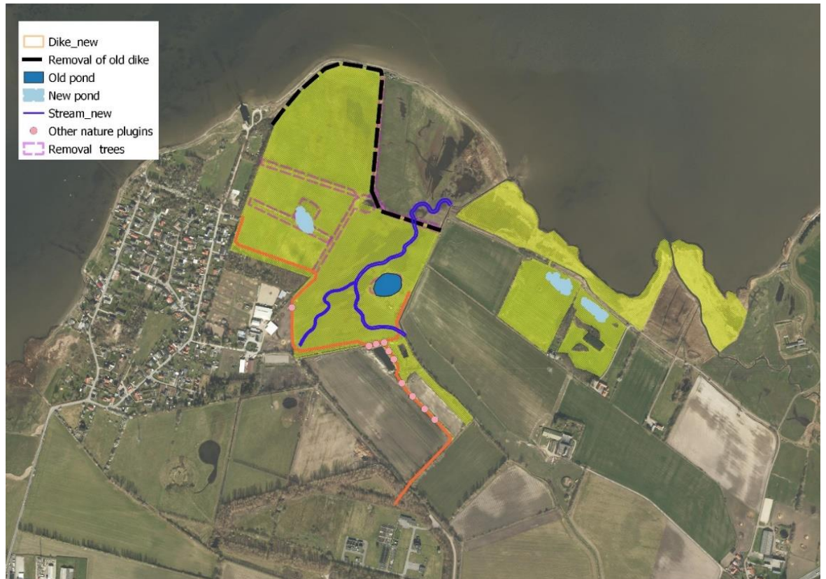
Figure 4-2: Visualization of the works done in the Seden Strand project (from Odense Municipality), including the placement of the relocated dike, the new meanders of the restored stream, the locations of new ponds and nature plug-ins.
