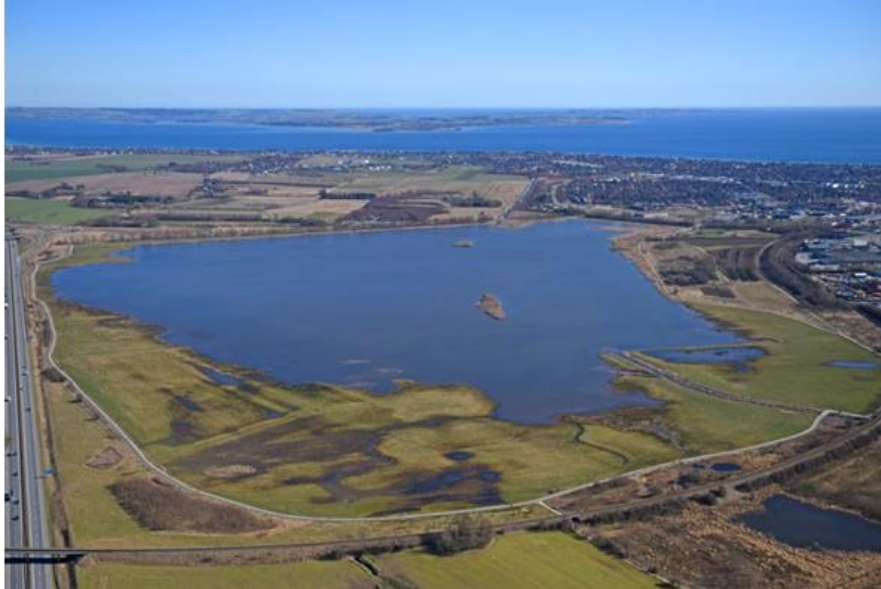
Figure 5-1: Lake Egå surrounded by grazed meadows. The purpose of establishing this wetland was to reduce the nitrogen supply to Aarhus Bay (in the background), to improve the natural conditions in and around the area, and to reduce the flood risk from the river Egå (from Deliverable 2.3 - Scope of Works for Demonstrators A and B).
